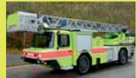
Turntable ladder ADL 2000 For rescue operations, recovering the injured, outside firefighting efforts and other operations from high up
