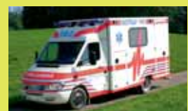
City of Zurich ambulance Sprinter 416 CDI, with case-shaped body, for emergency operations as well as patient and special transport
