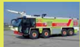
Airfield firefighting vehicle Z8 Up to 1,000 HP and 40 tons for fighting aircraft fires
